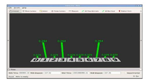
Now let's incorporate into our analysis the fact that the robot can move along the corridor. For that purpose, let's move the robot one grid cell per step to the right side. How does it change our belief? Let's consider our robot's odometry is perfect.
